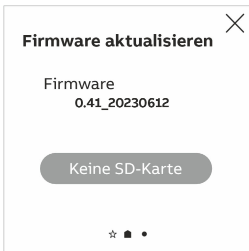
Fig. 37: Firmware update via SD card
